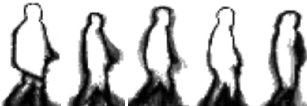
Figure 2.1: Several examples of GEnI, computed over a gait cycle. The gray level represents the entropy value in a pixel (x, y) . As can be seen, legs and arms have high gait entropy value, whereas static areas as torso have low values of entropy.
