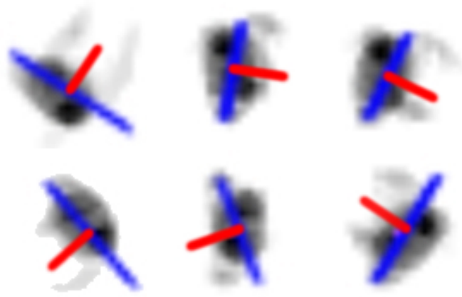
Figure 4.3: The displacement vector (red line) of the individual is computed at each time. The principal axis (blue line) is perpendicular to the displacement vector.
